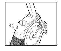
tabs at the front and along the sides of the Top Shield (44). Then, slide the Top Shield upward.
